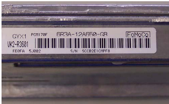
Fig 1: Part No. Located above the Bar Code ( ____-12A650-____)
